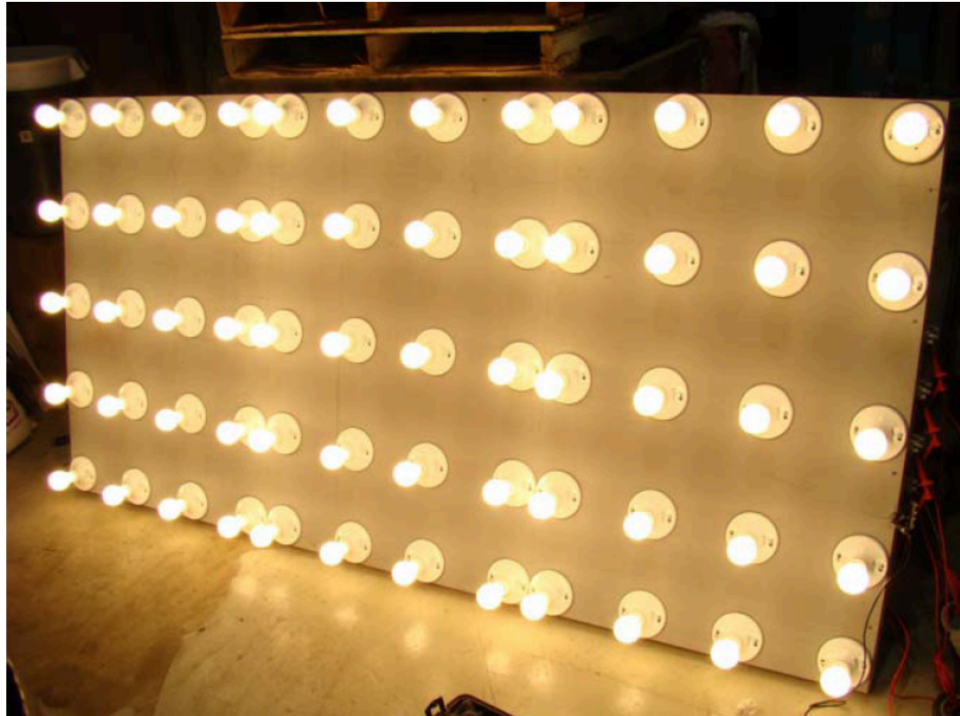
Figure 13 – Light Board used to generate harmonics 22
