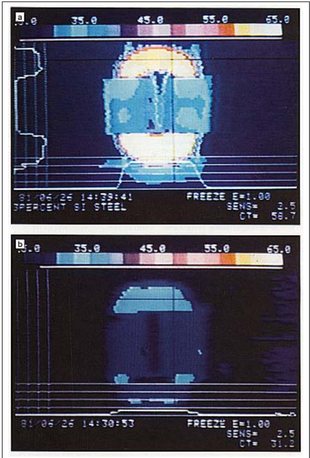
Figure 5 . Infrared photographs of (a) grain-oriented steel and (b) amorphous-metal distribution transformer core-coil assemblies.
