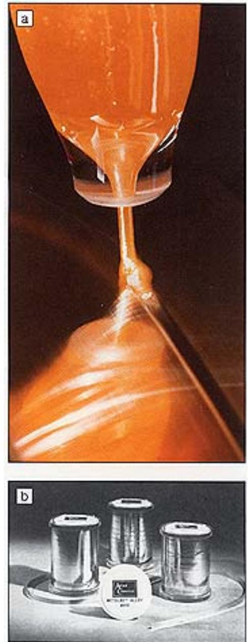
Figure 2(a) Chill block melt spinning by free-jet casting. (b) Free Jet Cast amorphous metal ribbon.
