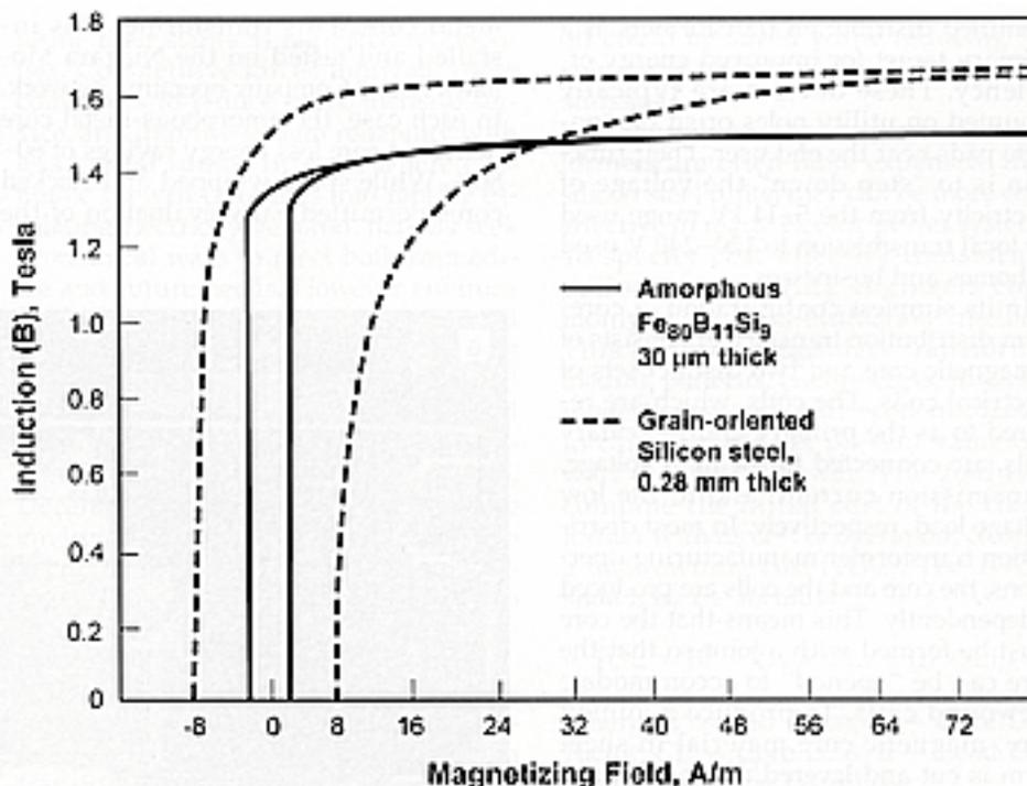
Figure 4. B-H characteristics of amorphous  $\text{Fe}_{80}\text{B}_{11}\text{Si}_9$  and grain-oriented silicon steel
